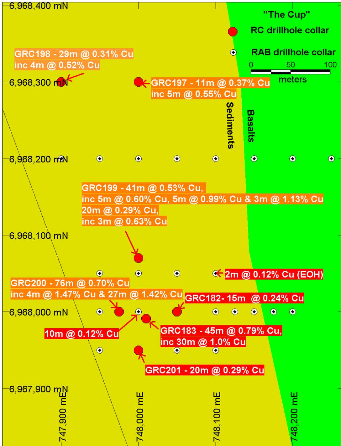
Drilling plan and significant results, The Cup (intersections calculated on 0.1% and 0.5% copper downhole cutoffs, orange text boxes are intersections from 1m split reassays, red boxes show previously announced results)
