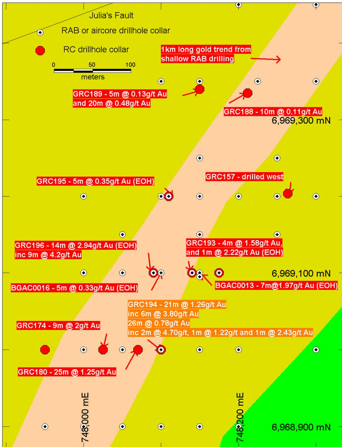
Drilling plan and significant results, Julia's Fault (intersections calculated at 0.1g/t and 1g/t gold downhole cutoffs orange text boxes are intersections from 1m split reassays, red boxes show previously announced results)
