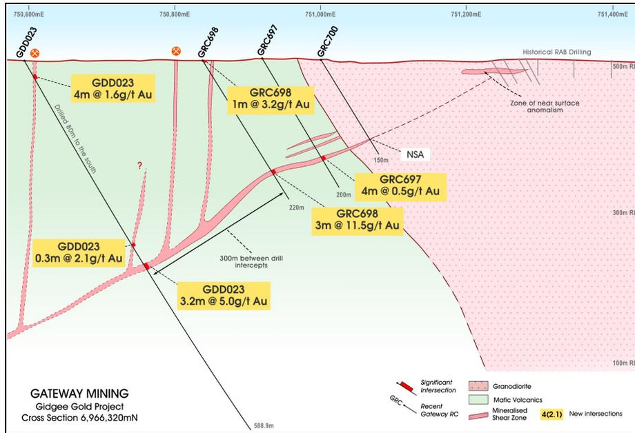
Figure (4): RC drill cross-section 6,966,320mN. Note hole GDD023 has been projected from 80m south.
