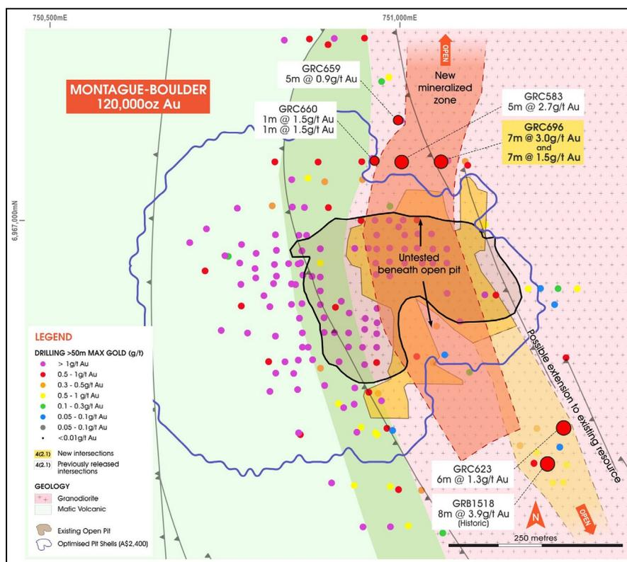
**Figure (2): Montague-Boulder Mineral Resource area RC drilling with new significant intercepts (yellow labels) and previous announced and historic intersections within the granodiorite proximal to the Mineral Resource (white labels). Note the AUD\$2,400/oz optimised shell which constrains the current Mineral Resource.**
