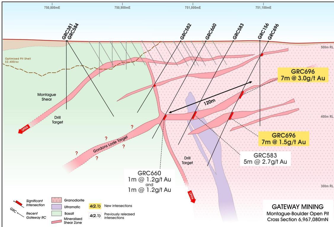
Figure (3): RC drill cross-section 6,967,080mN. Note the proximity of this new structure to the existing Mineral Resource interpretation and AUD\$2,400/oz optimal shell that constrains this Resource.
