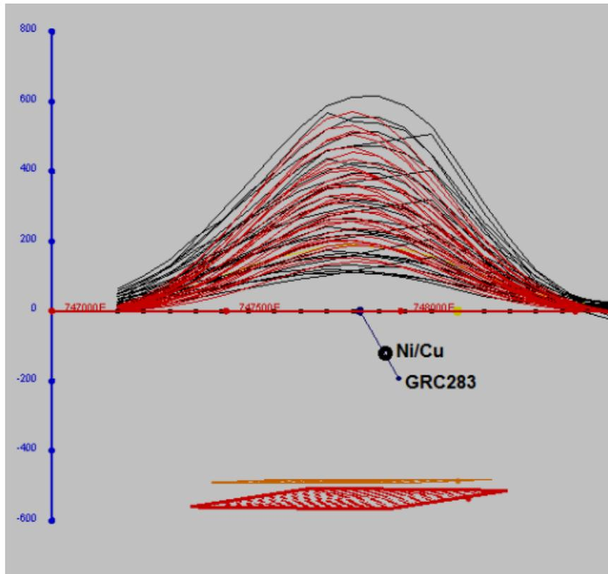
*Ni-Cu-PGE intersection relative to subsequently identified strong FLTEM conductor*
