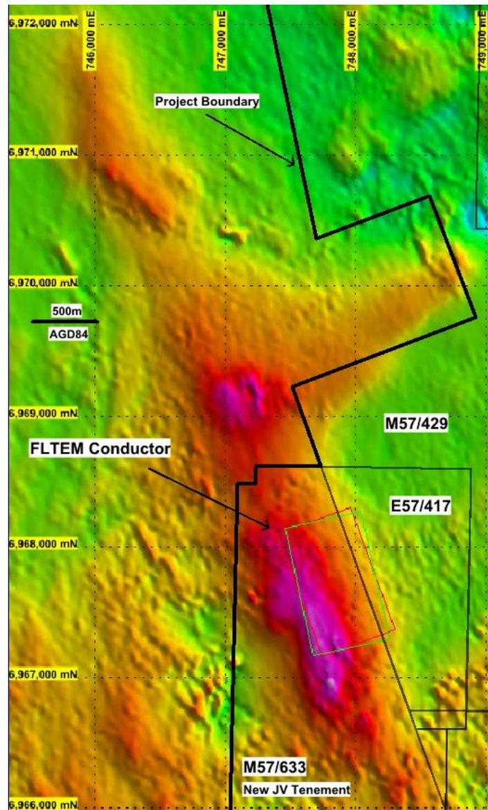
*FLTEM conductor relative to interpreted intrusion*
