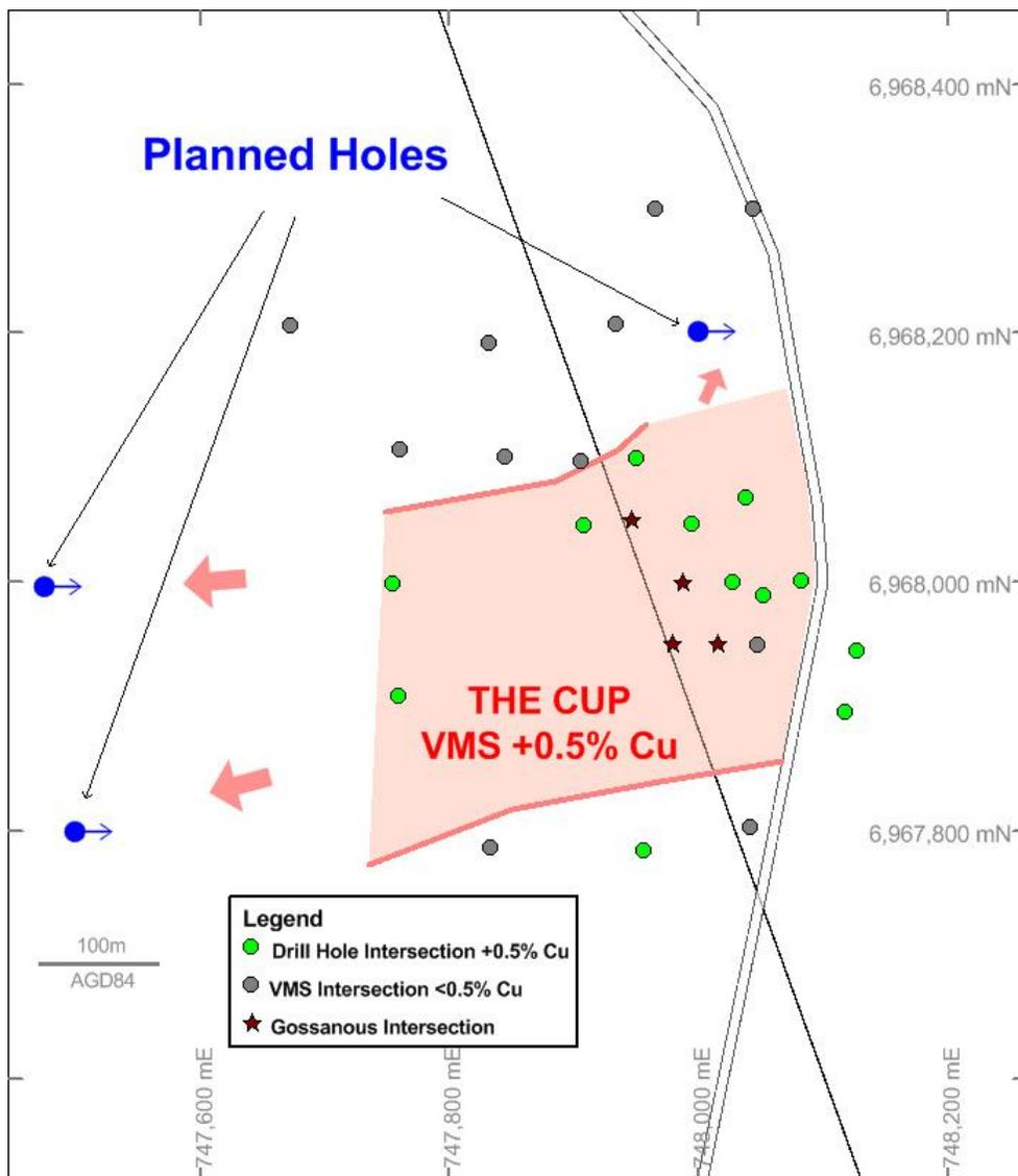
Plan view of drill holes at The Cup
