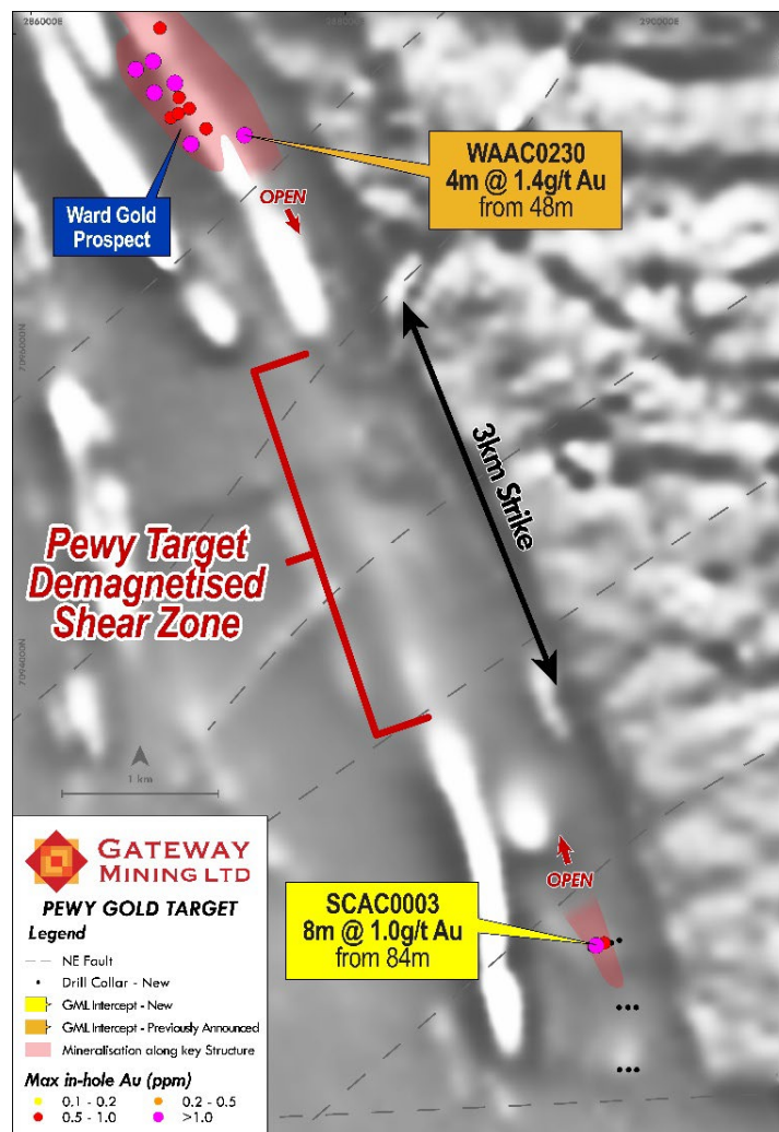
Figure 5: Demagnetised portion of the shear, highlighting Pewy.
