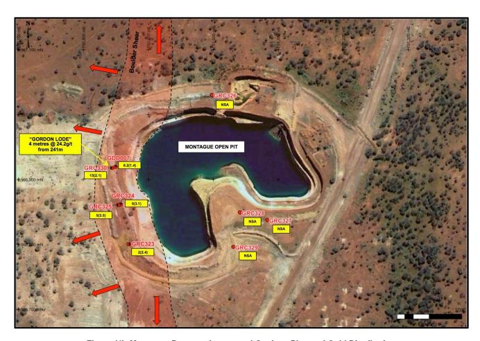
Figure (4): Montague Prospect Interpreted Geology Plan and Gold Distribution
