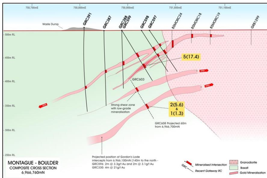
**Figure 2. Montague-Boulder Deposit – Indicative cross-section of typical mineralisation**
