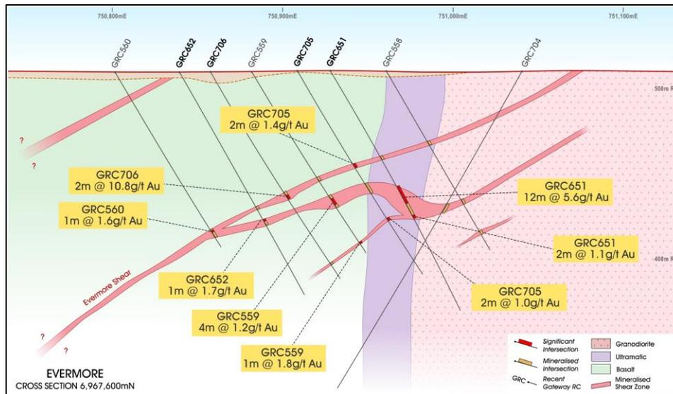
**Figure 3. Evermore Deposit – Indicative cross-section of typical mineralisation**
