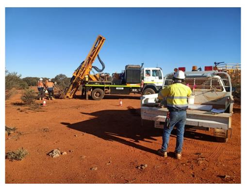
Figure (1): Air-core drill rig on site at the Plymouth North target.
