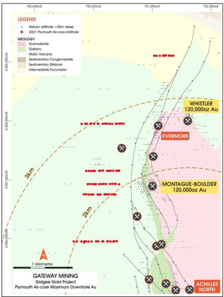
Figure (2): Plymouth air-core drilling hole location diagram.
