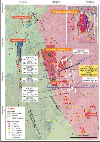
Figure (6): Plan view of the Achilles East target area. Note the proximity of the existing Achilles North oxide Mineral Resource. Inset plan view of the 120,000oz Whistler deposit at the same scale.
