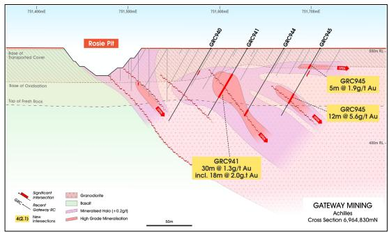
Figure (7): Achilles East cross-section B-B' illustrating previously intersected wide, east-dipping mineralisation in the Montague Granodiorite.
