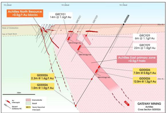
Figure (5): Cross Section A-A' corresponding to the trace of GRD026. Note the wide zones of east-dipping mineralisation within the Montague Granodiorite.
