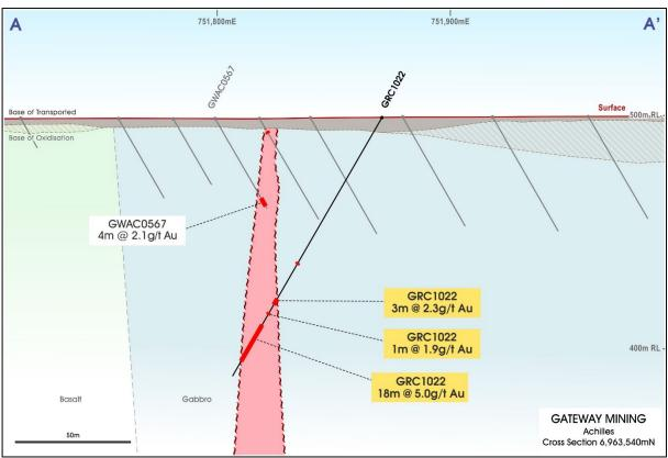
Figure (4): RC cross-section 6,963,540mN highlighting recent RC drill results at depth below anomalous aircore drilling in the transition zone.
