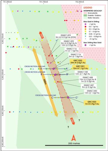
Figure (3): Duplex target with recently completed RC drilling and existing air-core drill coverage.
