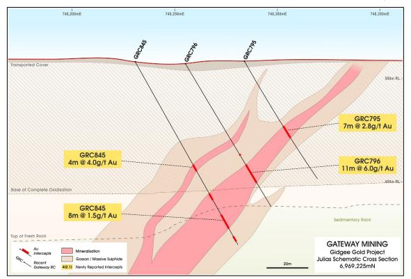
Figure (4): Julias in-fill RC drilling cross-section 6,969,225mN. Note the shallow nature of mineralisation and depth of weathering, associated with stronger gold grades.
