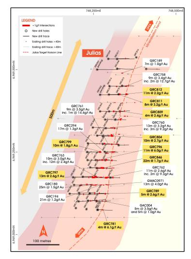
Figure (3): Julias deposit plan view, with recent significant intersections in RC drilling.
