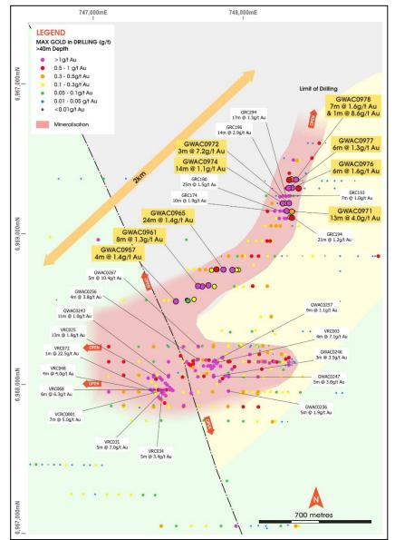
Figure (4): Julias air-core drilling maximum down-hole gold, with historic drilling >40m depth
