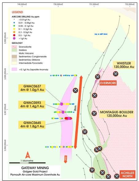
Figure (5): Plymouth air-core drilling maximum down-hole gold
