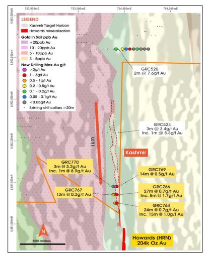
Figure (1): Kashmir RC drilling significant intercepts with interpreted geology on 2<sup>nd</sup> Vertical Derivative magnetics and proximity to the Howards deposit (ASX: HRN)
