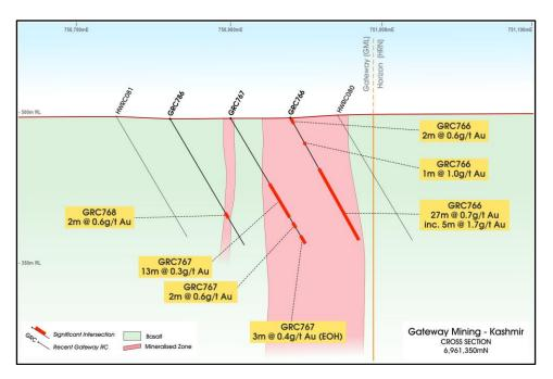
Figure (2): Kashmir RC drilling cross section 6,961,350mN
