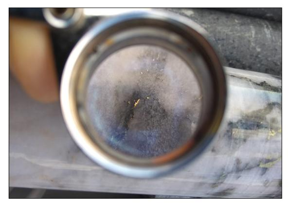
Figure (3): Visible gold observed in diamond drill core from hole GDD018, correlating to an interval of 1.9 metres @ 22.4g/t Au from 151.4m. Note hand lens 10x magnification.
