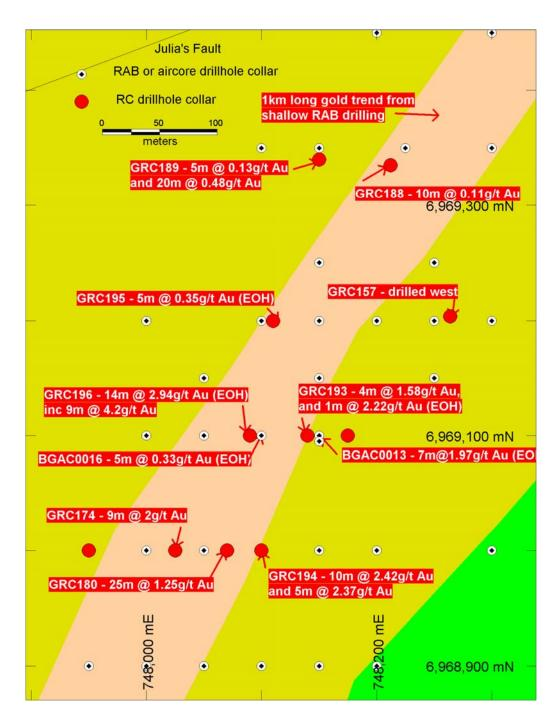
Drilling plan and significant results, Julia's Fault (intersections calculated at 0.1g/t and 1g/t gold downhole cutoffs)
