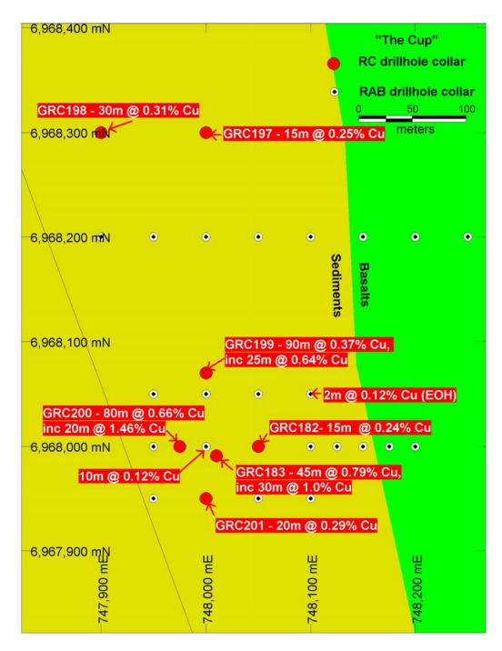
Drilling plan and significant results, The Cup (intersections calculated on 0.1% and 0.5% copper downhole cutoffs)
