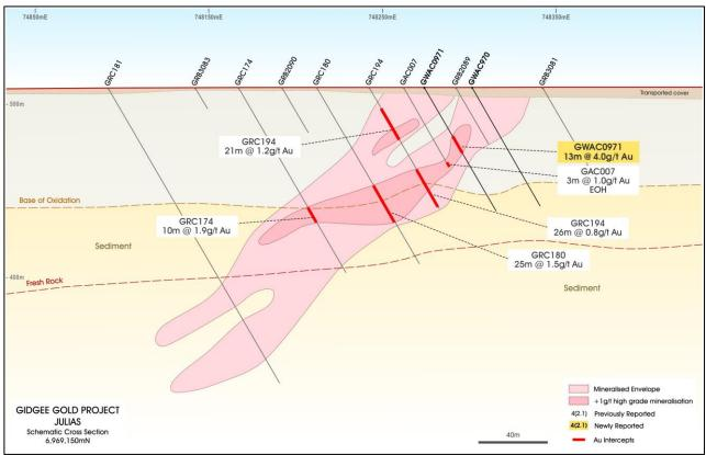
Figure (2): Julias air-core drilling cross section 6,969,150mN
