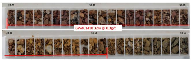
Figure (6): Plymouth north air-core hole GWAC1418 chip trays, illustrating the significant mineralised shear with quartz veining and remnant sulphides.
