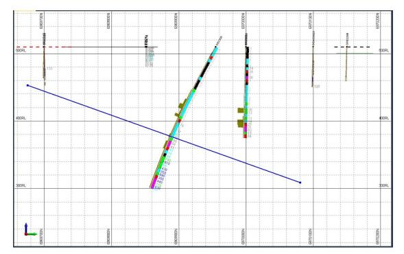
Cross section 748900E, Sulphide and gossan histogram, zinc assays, multielement colour trace
