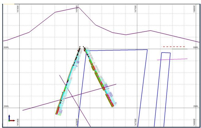
Cross section 6965300N, Sulphide and gossan histogram, zinc assays, multielement colour trace
