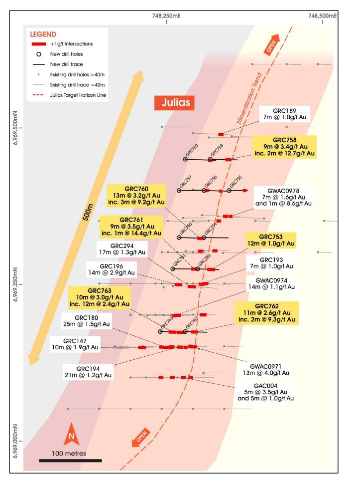
Figure (2): Enlargement of the core Julias target, with recent RC drilling significant intersections.
