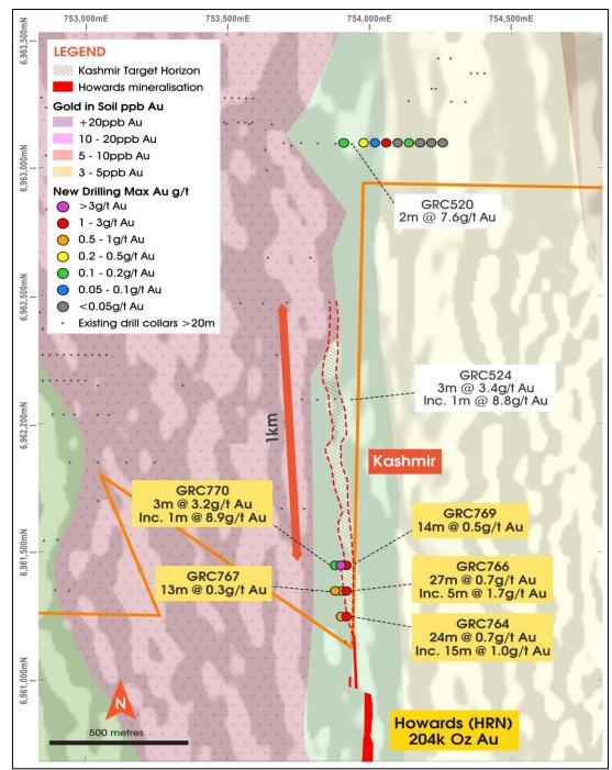
Figure (3): Kashmir RC drilling significant intercepts with interpreted geology on 2<sup>nd</sup> Vertical Derivative magnetics and proximity to the Howards deposit (ASX: HRN)
