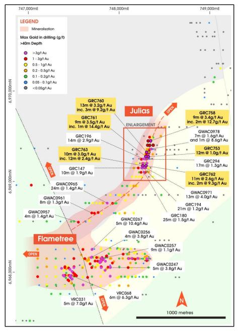
Figure (2): Julias-Flametree target areas with historic drilling and new RC results. Note the +2km corridor of shallow oxide mineralisation intersected to date
